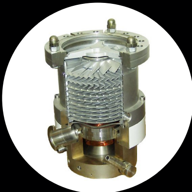
TMP: "interior view of a turbomolecular pump (TMP) - source: wikipedia
